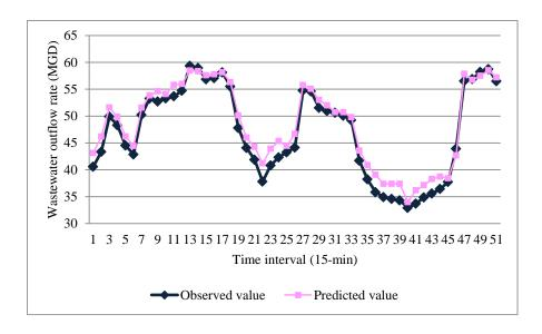
Figure 3.3. Observed and predicted wastewater outflow rates of C<sub>1</sub>
