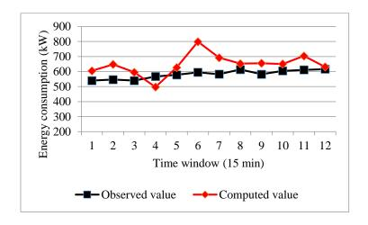
Figure 3.10. Computed and observe pump energy consumptions of CI2
