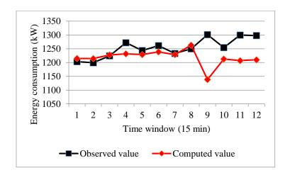
Figure 3.12. Computed and observe pump energy consumptions of CI3
