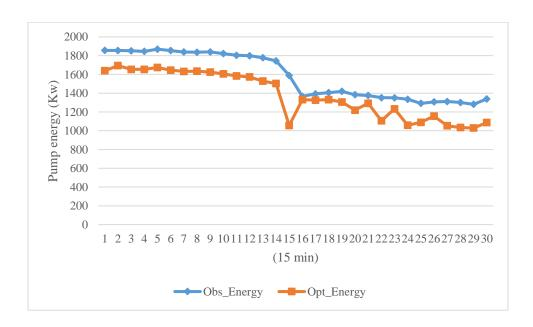
Figure 2.8. Observed and optimized pump energy consumption for scenario 3
