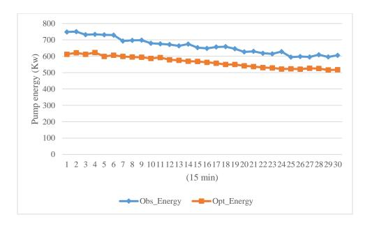
Figure 2.7. Observed and optimized pump energy consumption for scenario 2
