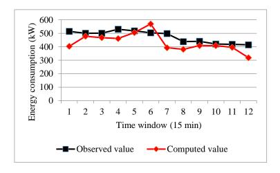
Figure 3.8. Computed and observe pump energy consumptions of CI1
