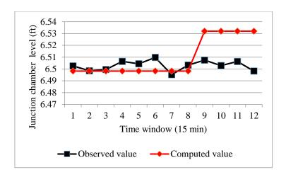
Figure 3.13. Computed and observed junction chamber levels of CI3
