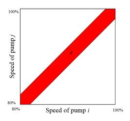
Figure 2.4. Optimization area of pump speeds for two pumps
