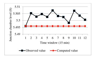
Figure 3.11. Computed and observed junction chamber levels of CI2
